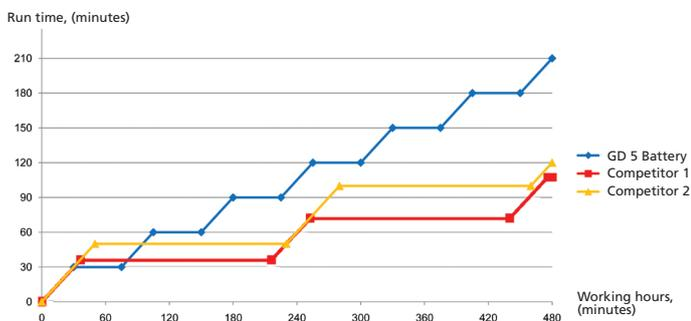
All horizontal lines indicated charge times for battery and diagonal lines show runtime.
