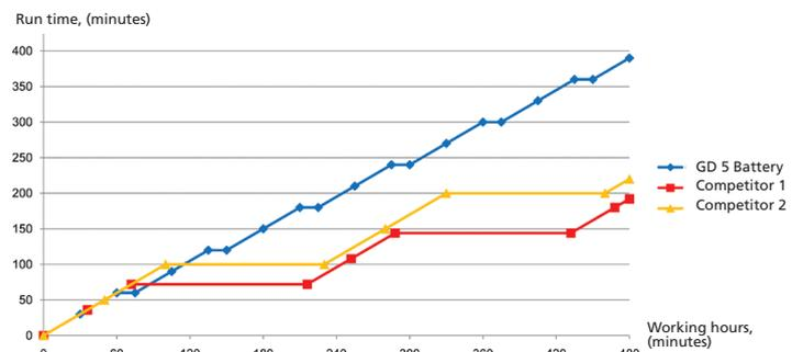
All horizontal lines indicate charge times for battery and diagonal lines show runtime.
